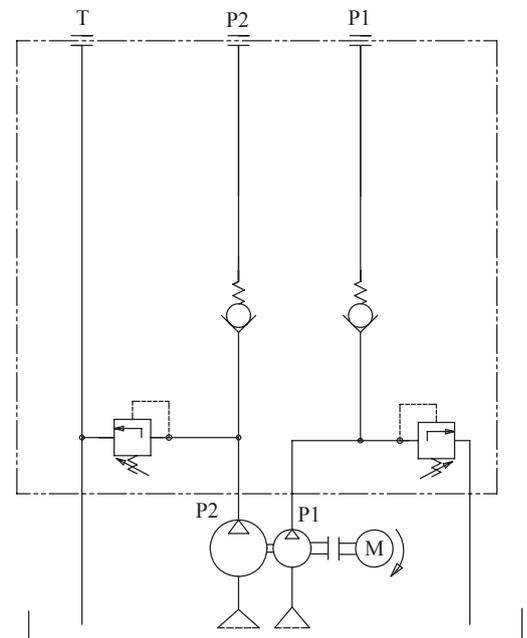
The W85A series power pack is designed for applications that need two independent hydraulic power supply, but only use a single A.C. motor.
